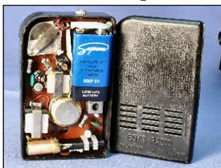
Another thing some importers did, that was new to the US market, was to introduce super low cost pocket radios with loudspeakers that would only pick up strong local AM radio stations. Almost all of these sets are identified on the back as "Boys Radio". Almost all of these radios
